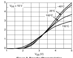
Figure 7. Transfer Characteristics
