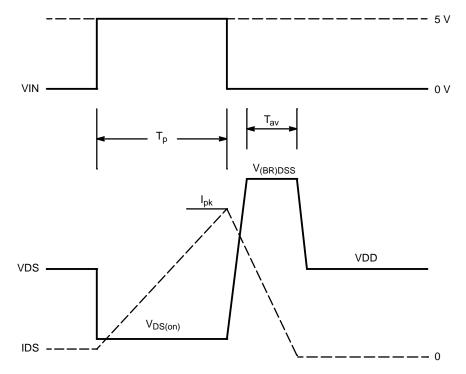
Figure 25. Inductive Load Switching Waveforms
