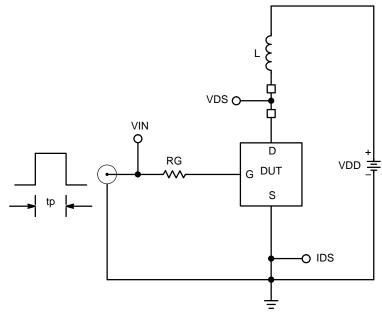
Figure 24. Inductive Load Switching Test Circuit
