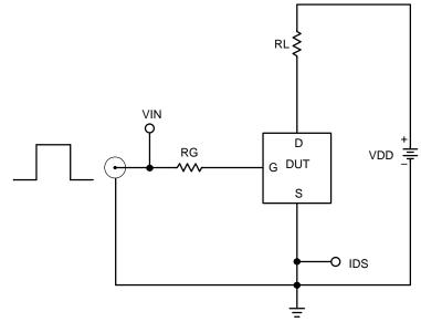
Figure 22. Resistive Load Switching Test Circuit
