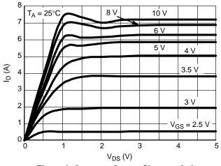
Figure 6. On-state Output Characteristics
