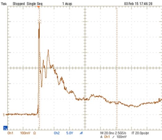
Figure 1. IEC61000-4-2 +8kV Contact ESD Clamping Voltage
