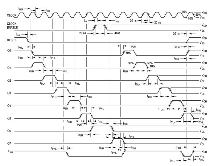
Figure 4. AC Measurement Definition and Functional Waveforms
