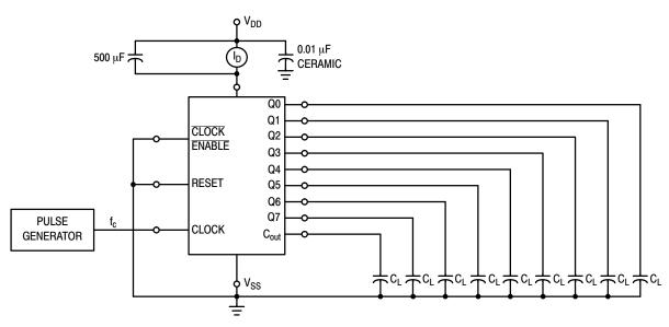
Figure 2. Typical Power Dissipation Test Circuit
