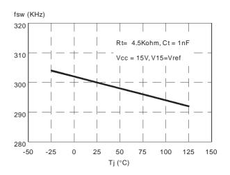
Figure 15. Switching frequency vs. temperature.
