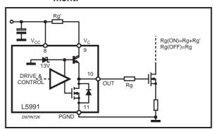
**Pin 10.** OUT (Driver Output). This pin is the output of the driver stage of the external power switch. Usually, this will be a PowerMOS, although the driver is powerful enough to drive BJT's (1.6A source, 2A sink, peak).
