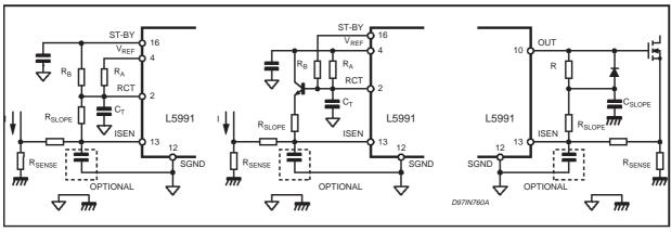
Figure 41. Protection against overvoltage/feedback disconnection (latched)
