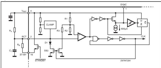
Figure 22. Oscillator and synchronization internal schematic.
