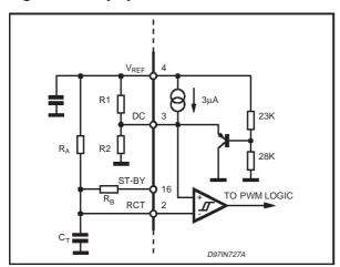
**Pin 4.** VREF (Reference Voltage). The device is provided with an accurate voltage reference (5V±1.5%) able to deliver some mA to an external circuit.
