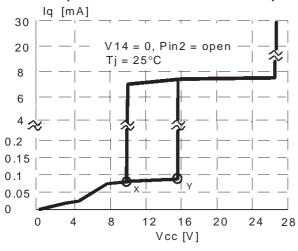
Figure 2. L5991 - Quiescent current vs. input voltage (after disable). (X = 7.6V and Y= 8.4V for L5991A)
