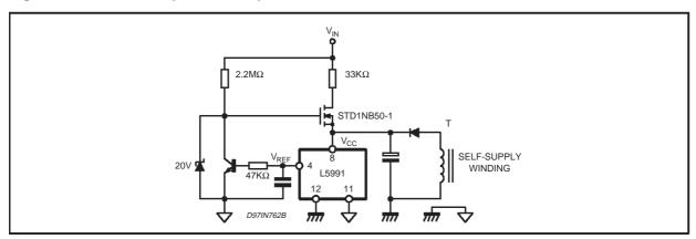
Figure 37. Bipolar transistor driver.
