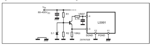
Figure 47. Synchronization to flyback pulses (for monitors).
