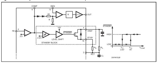
now disconnected and  $C_T$  is charged through  $R_A$  only. In this way the oscillator frequency ( $f_{SB}$ ) will be lower. Refer to pin 2 description to see how to calculate the timing components.
