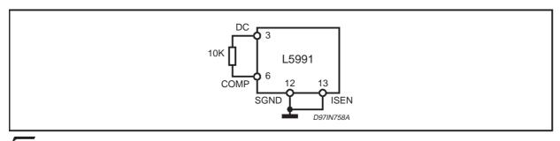
Figure 46. Device shutdown on mains undervoltage.
