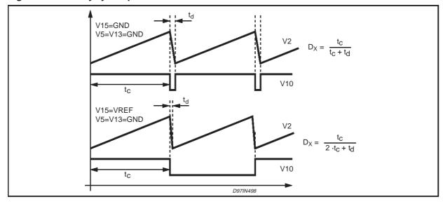
Figure 31. Standby function internal schematic and operation.
