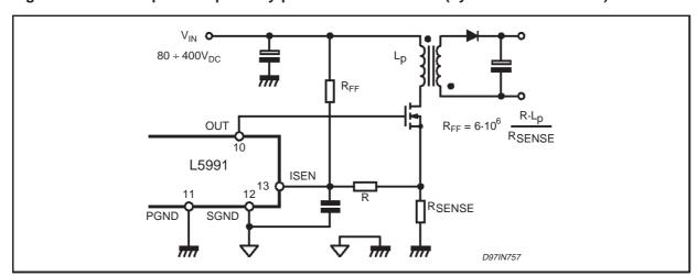
Figure 45. Voltage mode operation.
