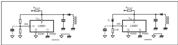
Figure 42 Protection against overvoltage/feedback disconnection (not latched)
