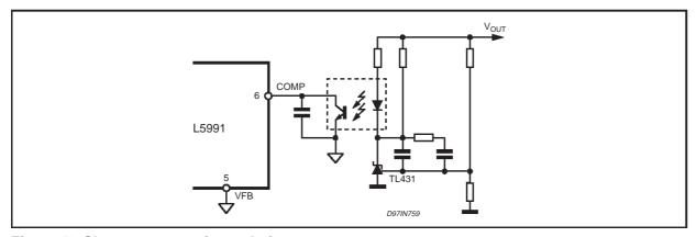
Figure 40. Slope compensation techniques.
