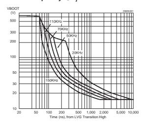
Figure 8.  $V_{boot}$  pin SOA @  $T_j = 125$ °C
