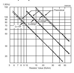
Figure 7.  $V_{boot}$  pin SOA for different Operating Frequency @  $T_i = 125^{\circ}C$
