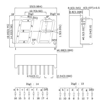
1. All dimensions are in millimeters (inches), Tolerance is  $\pm 0.25 (0.01")$  unless otherwise noted. 2. Specifications are subject to change without notice.
