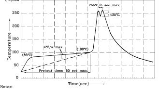
I.Recommend pre-heat temperature of 105°C or less (as measured with a thermocouple attached to the LED pins) prior to immersion in the solder wave with a maximum solder bath temperature of  $260^{\circ}$ C 2.Peak wave soldering temperature between  $245^{\circ}$ C ~  $255^{\circ}$ C for 3 sec
