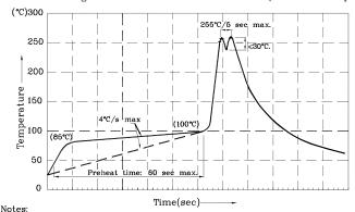
Notes. I. Recommend pre-heat temperature of 105°C or less (as measured with a thermocouple attached to the LED pins) prior to immersion in the solder wave with a maximum solder bath temperature of  $260^{\circ}C$  2. Peak wave soldering temperature between  $245^{\circ}C \sim 255^{\circ}C$  for 3 sec
