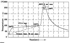
Notes: 1.Recommend pre-heat temperature of 105°C or less (as m thermocouple attached to the LED pins) prior to immersion wave with a maximum solder bath temperature of 260°C 2.Peak wave soldering temperature between 245°C ~ 255°C
