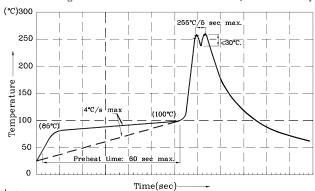
Notes: Notes. I. Recommend pre-heat temperature of 105°C or less (as measured with a thermocouple attached to the LED pins) prior to immersion in the solder wave with a maximum solder bath temperature of  $260^{\circ}C$  2. Peak wave soldering temperature between  $245^{\circ}C \sim 255^{\circ}C$  for 3 sec
