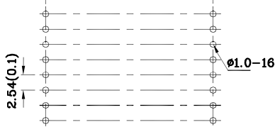
RECOMMENDED PCB LAYOUT 27.94(1.1)
