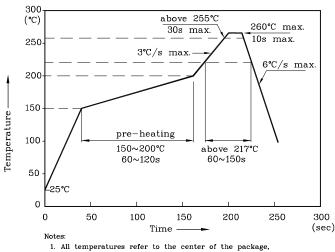
Reflow Soldering Profile for SMD Products (Pb-Free Components)
