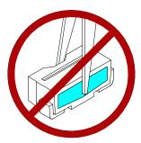
2. As silicone encapsulation is permeable to gases, some corrosive substances such as H<sub>2</sub>S might corrode silver plating of leadframe. Special care should be taken if an LED with silicone encapsulation is to be used near such substances.
