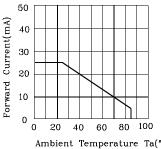
Ambient Temperature Ta(°C) FORWARD CURRENT DERATING CURVE
