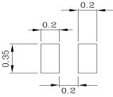
Mask open area ratio:80% Mask thickness:80~100um
