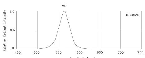
wavelength  $\lambda$  (nm) RELATIVE INTENSITY Vs. WAVELENGTH
