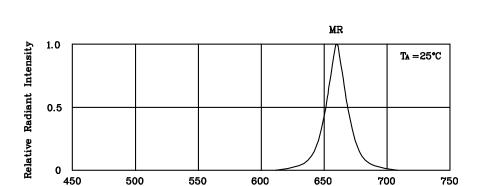
wavelength  $\lambda$  (nm) RELATIVE INTENSITY Vs. WAVELENGTH
