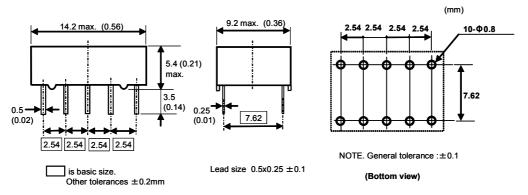
NJ type: Cover height 6.3mm, Lead length 2.8mm
