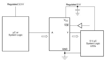
Figure 4. Typical Application Schematic
