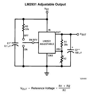
Note: Using 27k for R1 will automatically compensate for errors in V<sub>OUT</sub> due to the input bias current of the ADJ pin (approximately 1 µA).
