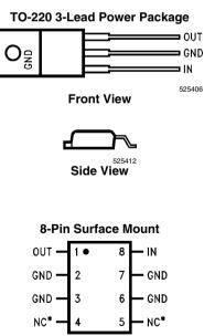
\*NC = Not internally connected. Must be electrically isolated from the rest of the circuit for the micro SMD package.
