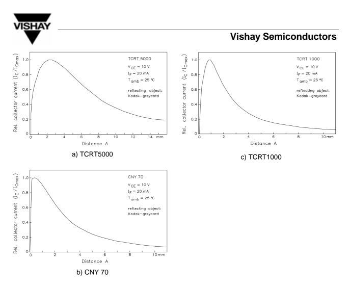
Figure 12. Working diagram of reflex sensors TCRT5000, CNY70 and TCRT1000
