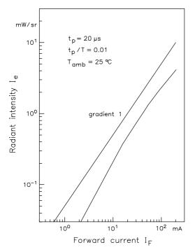
Figure 7. Radiant intensity,  $I_e = f(I_F)$ , of the IR transmitter
