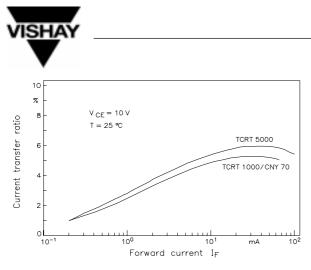
Figure 9. Coupling factor k = f(IF) of the reflex sensors
