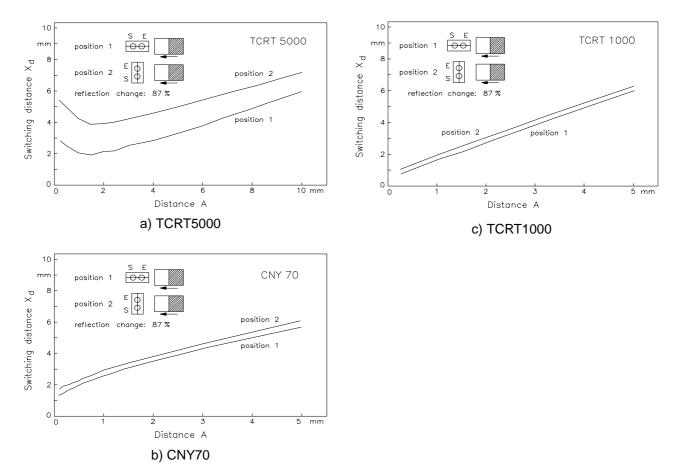
Figure 15. The switching distance as a function of the distance A for the reflex sensors TCRT5000, CNY70 andTCRT1000
