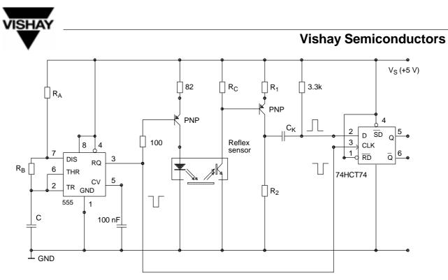
Figure 24. Pulse circuit with buffer storage
