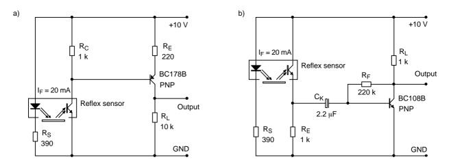
Figure 19. Circuits with transistor amplifier
