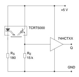
Figure 17. Reflex sensor - basic circuit
