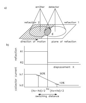
Figure 13. Abrupt reflection change with associated I<sub>c</sub> curve
