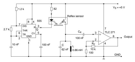
Figure 20. AC operation with oscillating circuit to suppress ambient light
