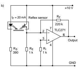
Figure 18. Circuits with operational amplifier
