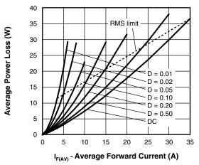
Fig. 6 - Forward Power Loss Characteristics
