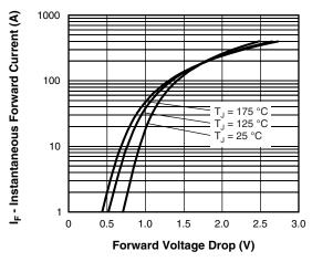
Fig. 1 - Maximum Forward Voltage Drop Characteristics (Per Diode)
