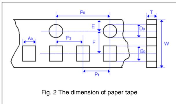
Fig. 2 The dimension of paper tape
