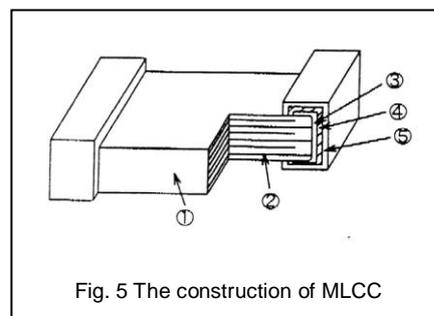
Fig. 5 The construction of MLCC
