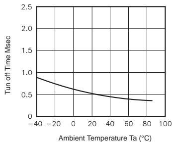
**Fig.5** LED operate vs. ambient temperature
