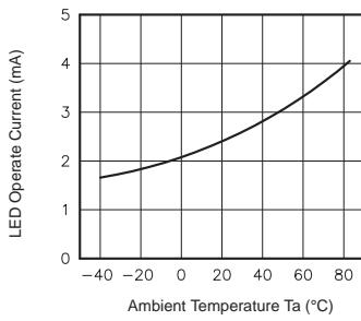
**Fig.6** LED turn off current vs. ambient temperature
