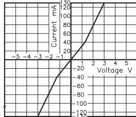
**Fig.9** Off state leakage current
