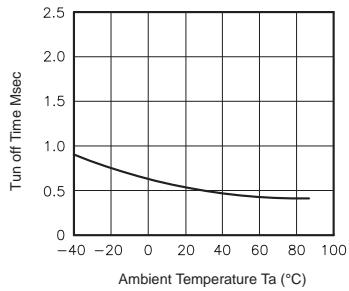
**Fig.5** LED operate vs. ambient temperature
