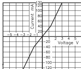
**Fig.9** Off state leakage current
