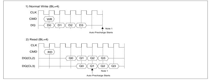
\* Note : 1. The row active command of the precharge bank can be issued after tre from this point. The new read/write command of other active bank can be issued from this point. At burst read/write with auto precharge, CAS interrupt of the same/another bank is illegal.
