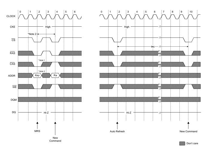
\* Both banks precharge should be completed before Mode Register Set cycle and auto refresh cycle.
