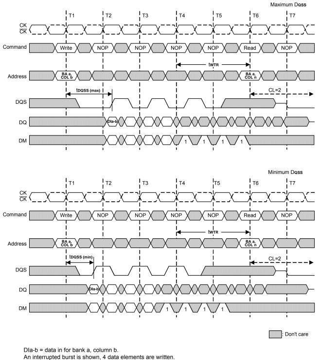
3 subsequent elements of data in are applied in the programmed order following DIa-b.
