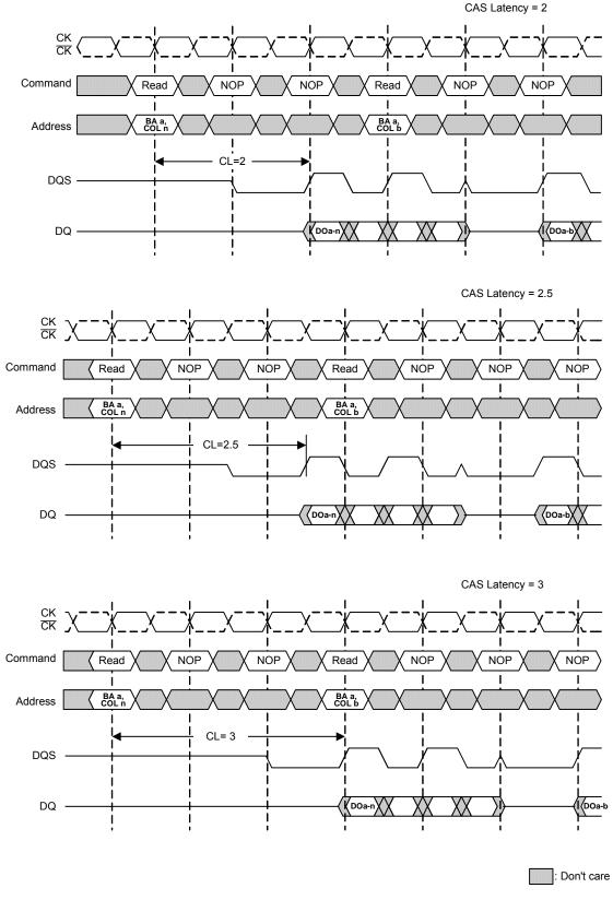
DOa-n (or a-b) = data out from bank a, column n (or bank a, column b). 3 subsequent elements of data out appear in the programmed order following DOa-n (and following DOa-b). Shown with nominal tac, tразск, and tраза.
