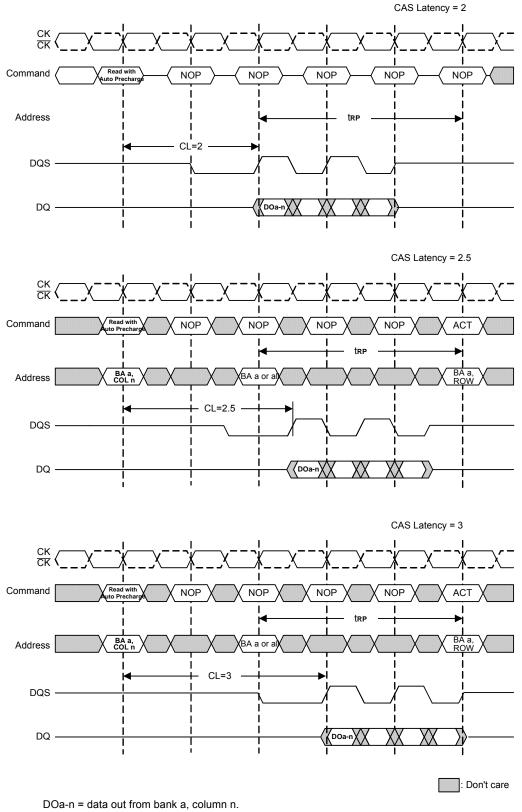
Cases shown are either uninterrupted bursts of 4 or interrupted bursts of 8.
