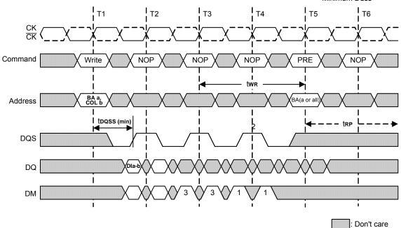
Dla-b = data in for bank a, column b. An interrupted burst is shown, 2 data elements are written.
