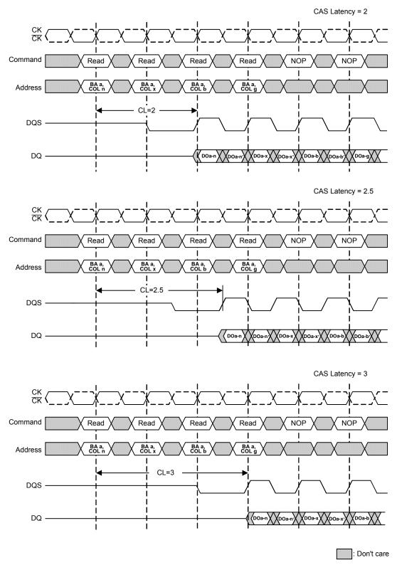
DOa-n, etc. = data out from bank a, column n etc. n' etc. = odd or even complement of n, etc. (i.e., column address LSB inverted). Reads are to active rows in any banks.
