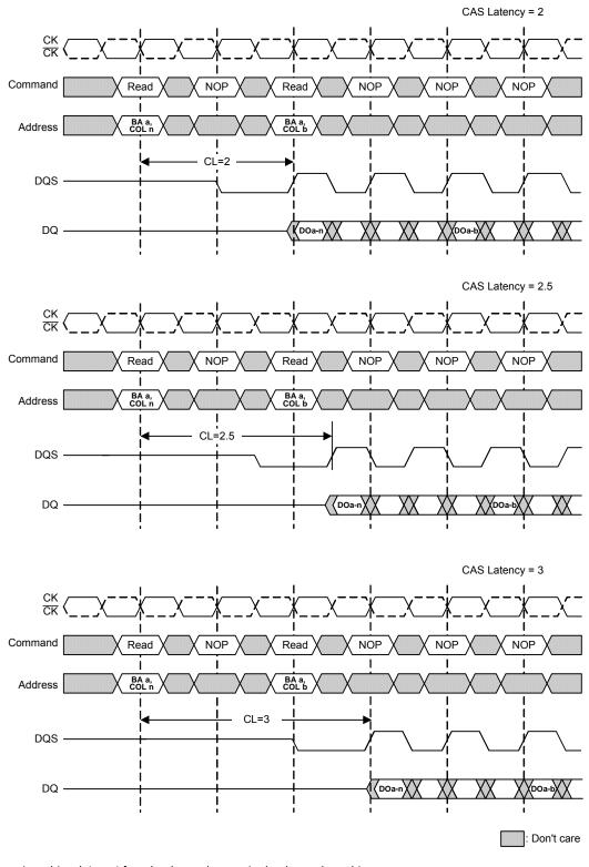
DOa-n (or a-b) = data out from bank a, column n (or bank a, column b). When burst length = 4, the bursts are concatenated. When burst length = 8, the second burst interrupts the first. 3 subsequent elements of data out appear in the programmed order following DOa-n. 3 (or 7) subsequent elements of data out appear in the programmed order following DOa-b. Shown with nominal tac, toosck, and tooso.
