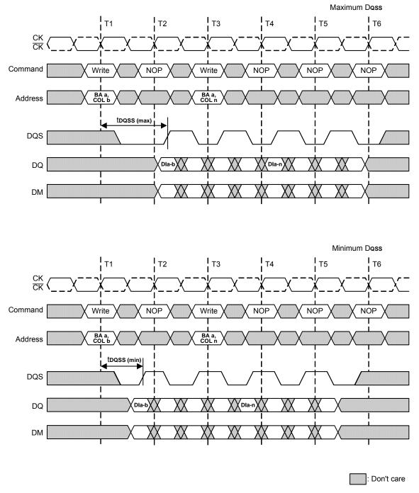
DIa-b = data in for bank a, column b, etc. 3 subsequent elements of data in are applied in the programmed order following DIa-b. 3 subsequent elements of data in are applied in the programmed order following DIa-n. A non-interrupted burst is shown. Each Write command may be to any bank.
