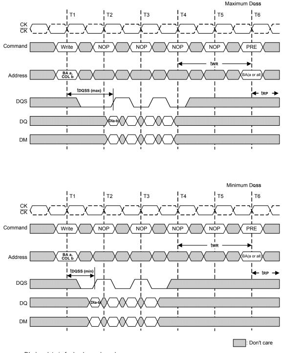
DIa-b = data in for bank a, column b. 3 subsequent elements of data in are applied in the programmed order following DIa-b. A non-interrupted burst is shown. two is referenced from the first positive CK edge after the last data in pair. A10 is Low with the Write command (Auto Procharge is disabled)
