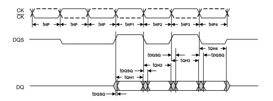
the is the half cycle pulse width for each half cycle clock. the is referenced to the clock duty cycle only and not to the data strobe (DQS) duty cycle.
