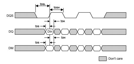
DIn = Data in for column n. 3 subsequent elements of data in are applied in programmed order following DIn.
