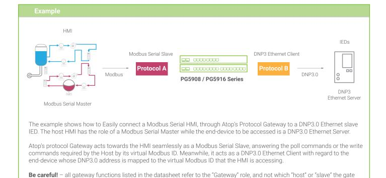
way is connected to. In this example, the SKU shown is "MBSS-DNEC" (Modbus Serial Slave to DNP3.0 Ethernet Client)
