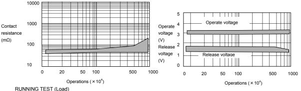
(Load: none, Drive:5VDC, 50Hz, 50%duty, Ambient temperature :room temperature, Sample:UA2-5NU ,20pieces)
