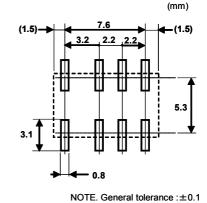
Tolerance of lead pitch is  $\pm 0.15$ mm (0.006inch) Other tolerances ±0.3mm (0.012inch)
