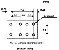
Tolerance of lead pitch is  $\pm 0.15$ mm (0.006inch) Other tolerances  $\pm 0.3$ mm (0.012inch)
